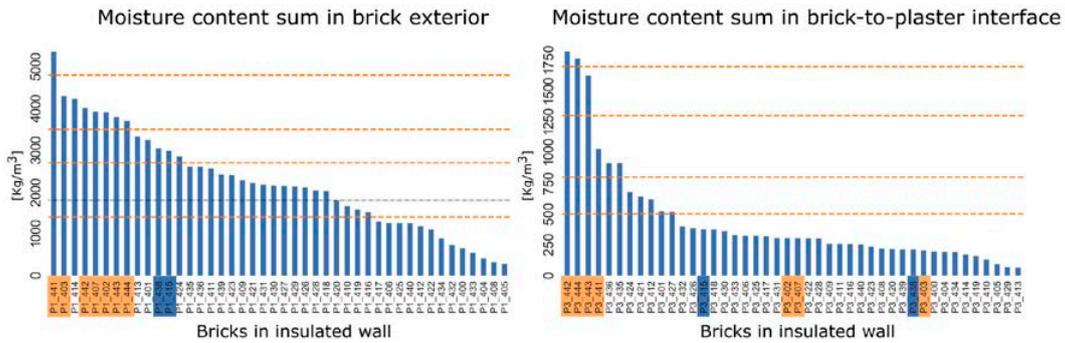
Figure 3. Ranking of bricks based on sum of moisture content at the exterior (left) and the brick-plaster surface (right) of an insulated 1½ brick thick SW oriented wall. Location Copenhagen, winter 2026–2027 (Dec 1 – Mar 1). Bricks marked with orange and blue boxes refer to the highest-ranking bricks in Figure 2.
